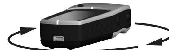
**NOTE:** The eTrex Vista must be held level during compass calibration and during use. The more the unit is tilted on either axis, the less accurate the compass readings will be.
